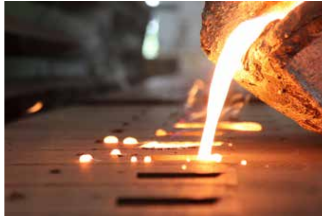
High temperature metal pouring into a casting mold.
