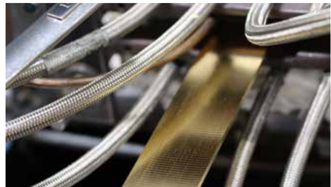
Gold strip going through the rolling machine.
