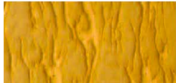
Typical microstructure of Silvar™ and Silvar-K™
