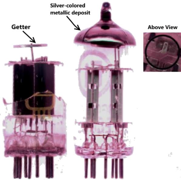
*From Wikipedia : A vacuum tube with a "flashed getter" coating on the inner surface of the top of the tube. (left) The inside of a similar tube, showing the reservoir that holds the material that is evaporated to create the getter coating. During manufacture, after the tube is evacuated and sealed, an induction heater evaporates the material, which condenses on the glass.*
